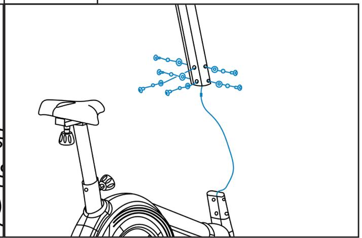
Connect the wires from the handlebar post to the main frame, making sure the pins are aligned and you hear a click. Then, secure the handlebar post to the main frame using six M8 hex socket head screws, six spring washers and six arc washers.
