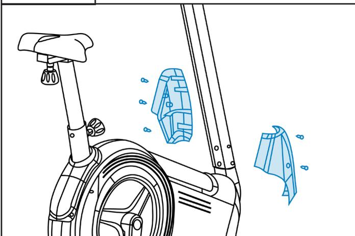
Remove the five tapping screws from the covers and slot around the post, then re-attach the screws to secure in place.
