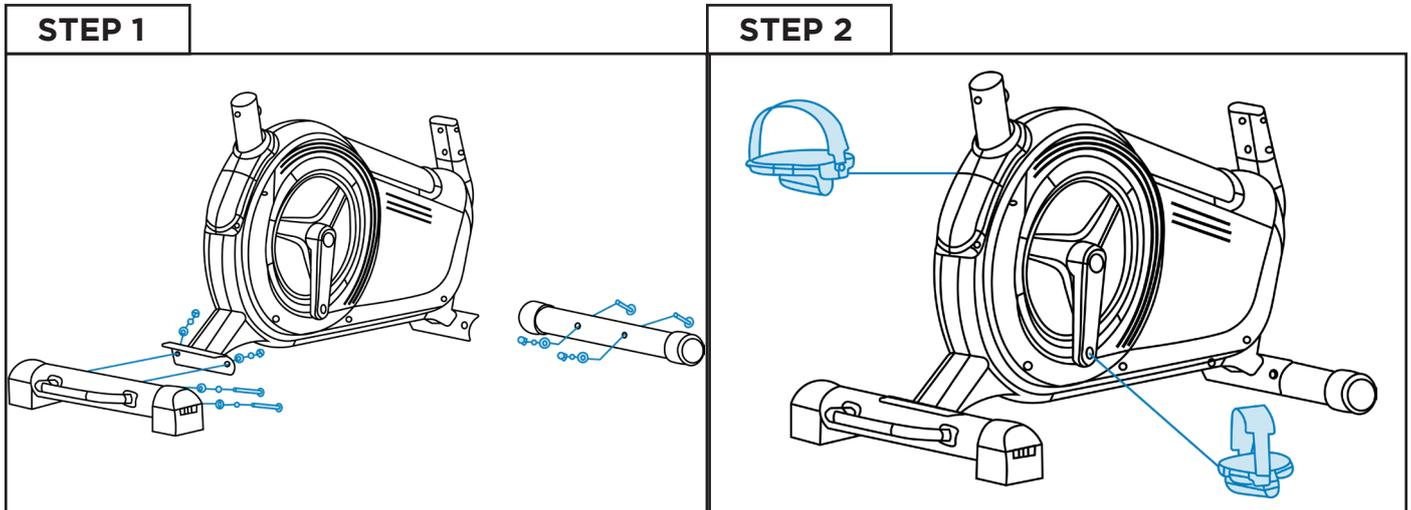
Attach the front and rear stabilisers to the main base using four M8 square neck bolts, four arc washers, four spring washers and four M8 domed nuts. Tighten using the multi-tool.
