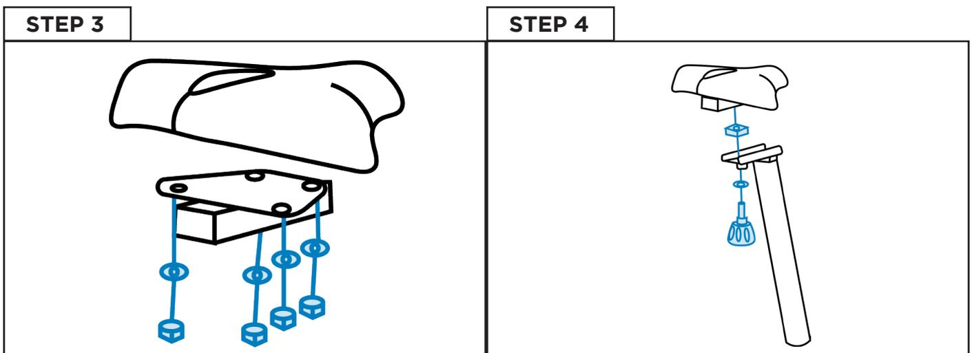
First attach the saddle to the horizontal seat post using four M8 hex socket head screws and four flat washers.
