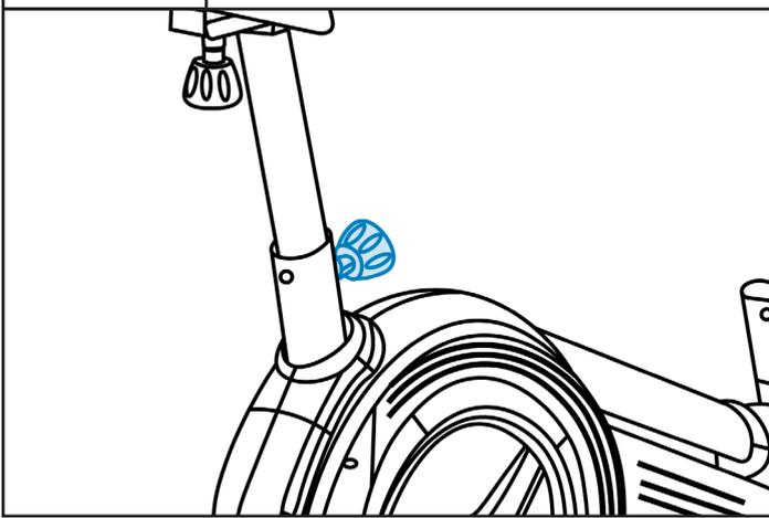
Slide the seat post into the main frame using another adjustment knob to lock it in place.
