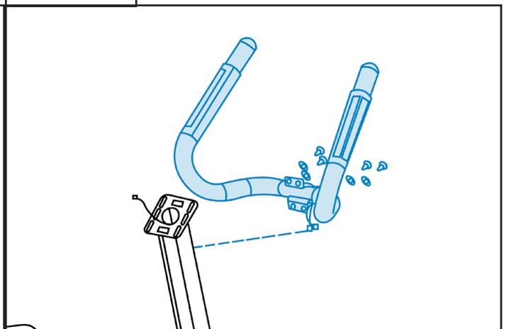
Thread the pulse wires from the handlebars through the back of the handlebar post and pull them up through the monitor bracket. Then, fix the handlebars using four M8 hex socket head screws and four flat washers.
