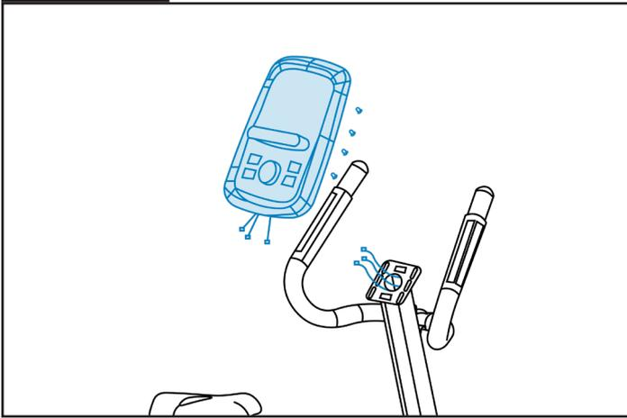
Connect the pulse wires from the handlebar post to the monitor, again making sure your pins are aligned. Then, secure the monitor to the bracket using the four screws found in the back of the monitor.
